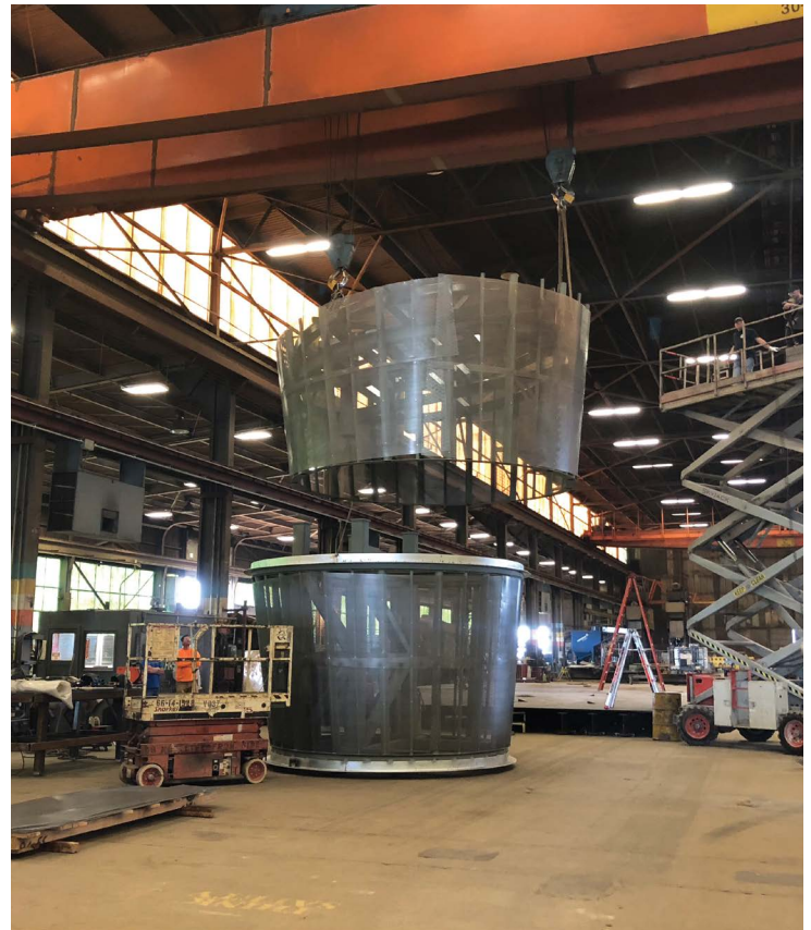
Kerry James Marshall's A Monumental Journey was engineered in three sections at Johnson Machine Works in Chariton, Iowa, then assembled on site in Des Moines. Photo: M. J. Rowe, 2018
